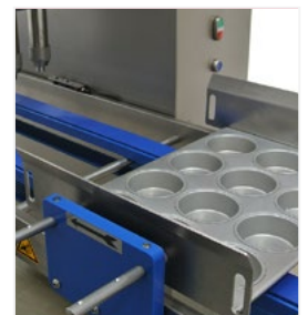
Conveyor belt with system to place trays of different sizes.
