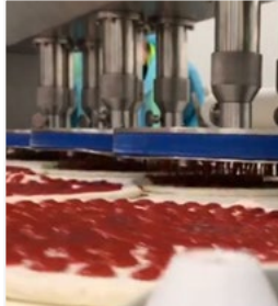
Nozzle with sprinkler outlet to spread tomato sauce into pizza base.
