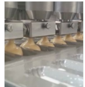
Double outlet doser to distribute the product into the moulds.
