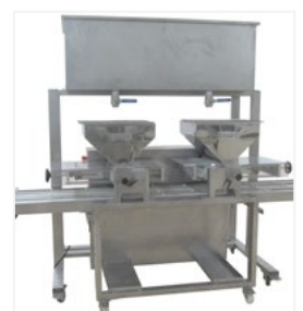
Double hopper to dose two colour doughs or different flavours.
