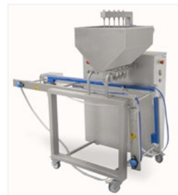
Model with folding conveyor belt to optimize storage.
