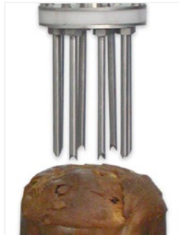
Large circular injector nozzle to fill panettone
