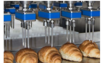
Triple injection nozzle for croissant fillings
