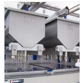
Double heated hopper to work with two flavours of fillings.
