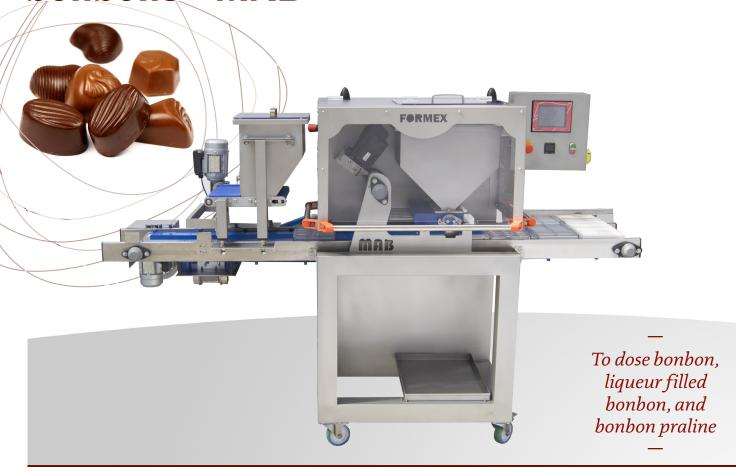
Filling machine for small doses suitable for chocolat production. It can dose: bonbon, liqueur filled bonbon, and bonbon praline. In the latter case the particles may reach up to 3 mm in diameter always depending on the density of particle concentration in chocolate.
